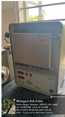
Wax Burnout Furnace
